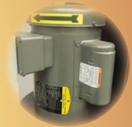
TEFC Motor and switch are fan-cooled and safe from dust-laden air stream
