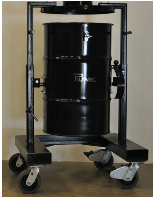
Cyclone cart has forklift pockets
