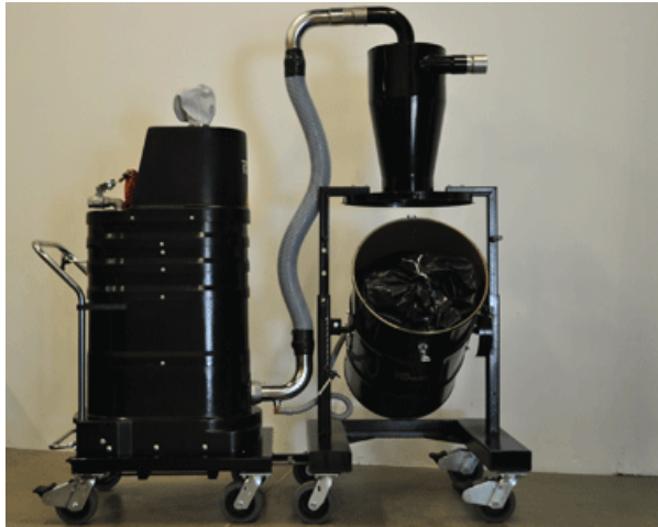
Drum locks in place to tie off waste liner
