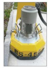
Features a Removable Side Door that enables this machine to polish and grind up against the edge!
