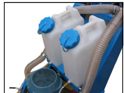
2 - 25ltr. Water Tanks for Wet Grinding
