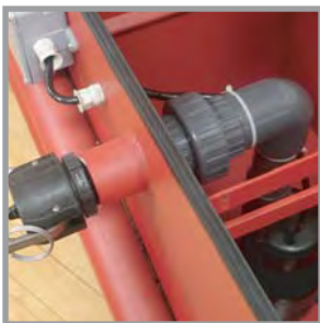
Return pump allows liquid return at 38 gallons/minute.
